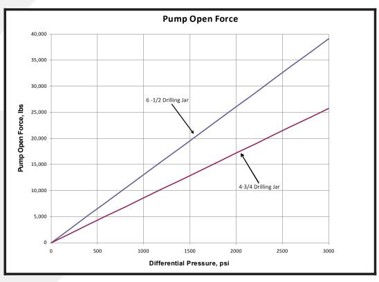
**Definition:** Pump open force is the force caused by the differential pressure between the jar bore and the annulus bore while circulating. It has the effect of pumping the tool open.
